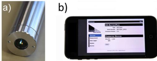
**Figure 3:** The multi-parameter fluorometer (a) shows the housing with illuminated LEDs and (b) shows the web interface how the devices can be controlled with the mobile end-device. Instrument and web interface is manufactured by TriOS (Germany).
