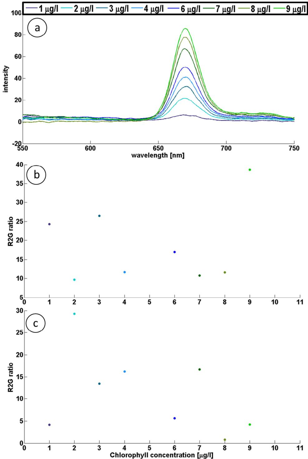
**Figure 5:** The results of the different measurement methods. Results of (a) the laboratory fluorometer are given as intensity versus wavelength. For (b) the measurement setup and (c) the prototype the results are given in R2G ratio versus Chl *a* concentration. The color code for (b) and (c) is as in (a).
