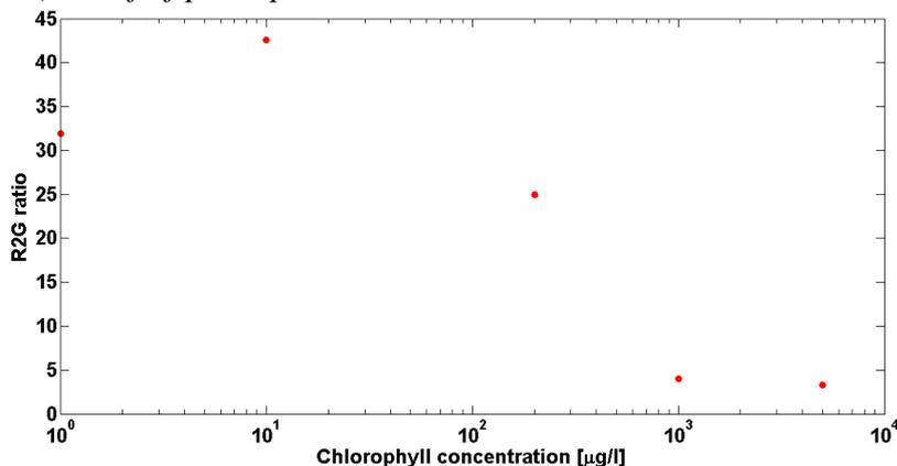
**Figure 4:** The R2G ratio for Chl *a* concentration 1  $\mu\text{g/l}$ , 10  $\mu\text{g/l}$ , 200  $\mu\text{g/l}$ , 1000  $\mu\text{g/l}$  and 5000  $\mu\text{g/l}$  are semi logarithmic presented. The data are derived with the measurement setup and a dilution series of Chl *a* standard.
