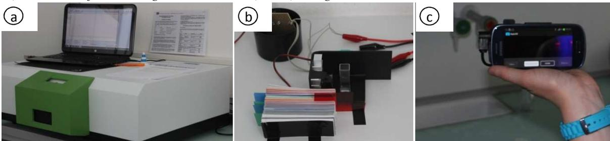
**Figure 2:** The three different measurement systems are shown (a) the laboratory fluorometer, (b) the measurement set up with the external LED and the external camera (not shown) as detector, and (c) the prototype of the smartphone adapter.
