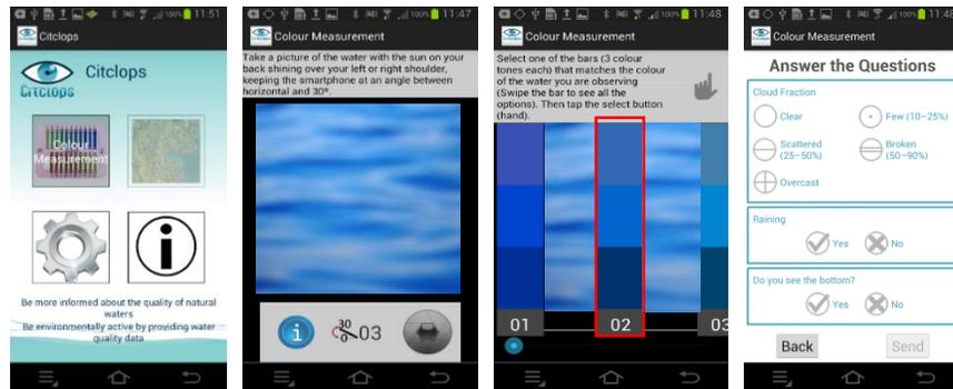
Figure 3. Smartphone application for the water color comparison. The observer takes a picture following the specified protocol, compares it to the FU digital scale, and then answers questions on the meteorological and location conditions.
