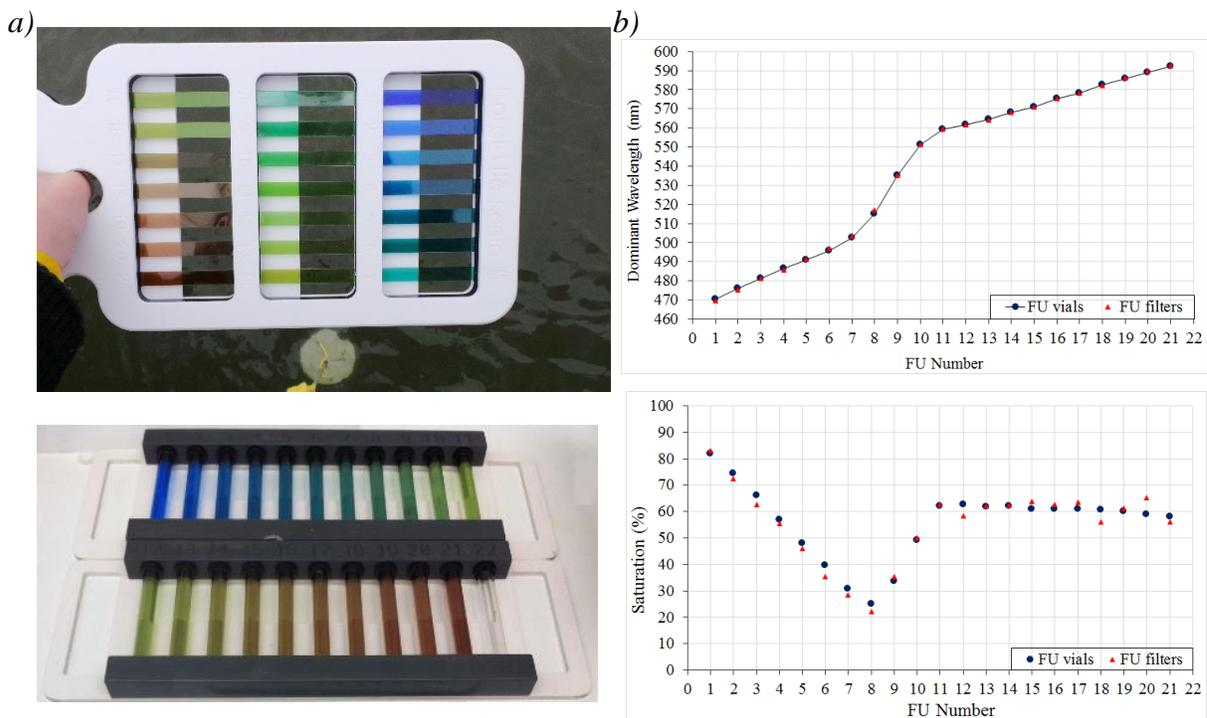
Figure 2 a) Picture of the resulting Modern FU scale, made of lighting filters, and the original FU liquid scale (bottom right). 2 b) Dominant wavelength and Saturation percentage, respectively, of the instrumentally measured vials and filter combinations.
