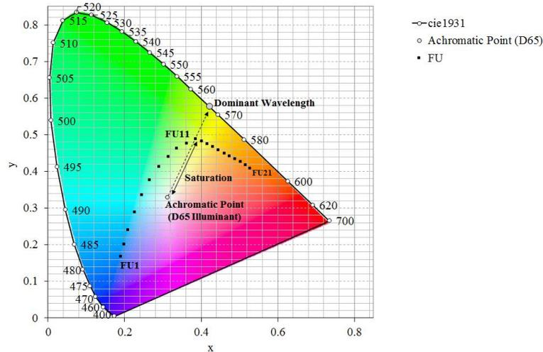
Figure 1. The CIE1931 chromaticity coordinates, based upon transmission measurements, of the FU-scale colours 1 to 21 (Novoa *et al.* 2013 (22)) including the achromatic point of a D65 illuminant. The outer curved boundary is the spectral locus, with wavelengths shown in nanometers.
