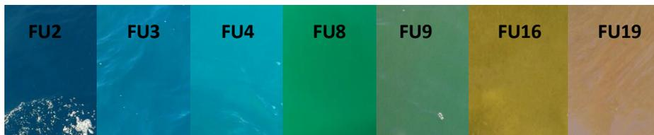
Figure 5. Example of images sent by the public, where FU index selected by the public in the digital scale matched the FU calculated by the algorithm.
