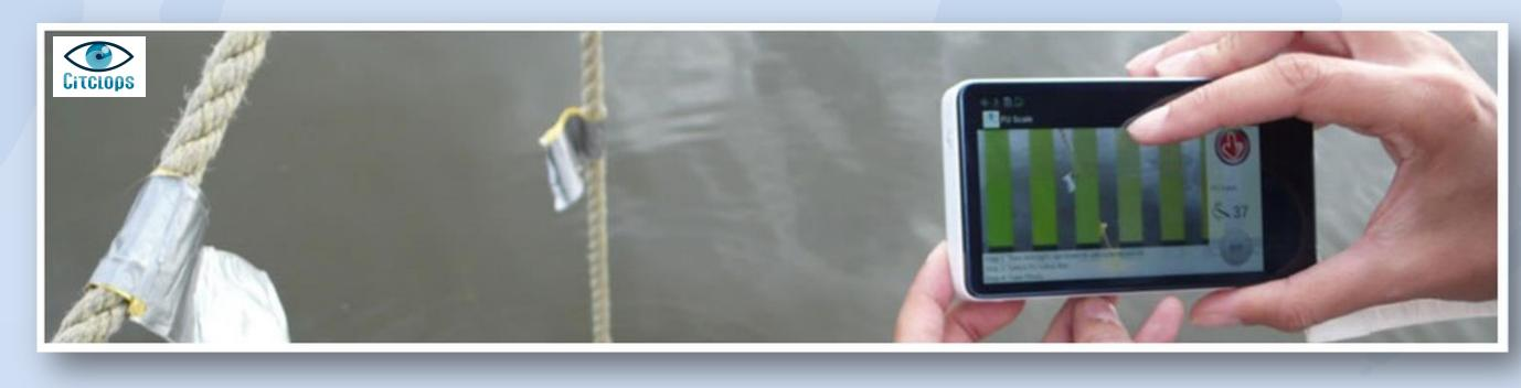
Citizens can help science by using the smartphone app, developed under the EU-project Citclops. An area of the sea can be selected on-screen and the colour of the water of this area can be compared with an on-screen Forel-Ule colour bar. Pictures and metadata are sent
